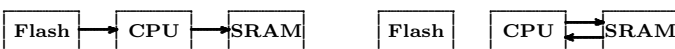
Fig.I: Booting of an embedded device. The Flash-ROM's contents are copied into SRAM, from where they are being executed afterwards.
