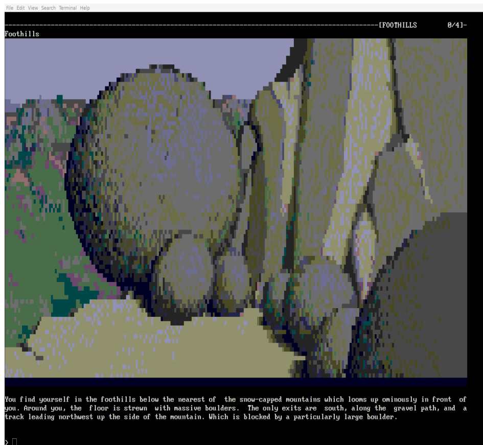
Figure 3.7: The utf mode offers a compromise between readable text, colours, and medium size resolution. It works in most terminal emulators.
